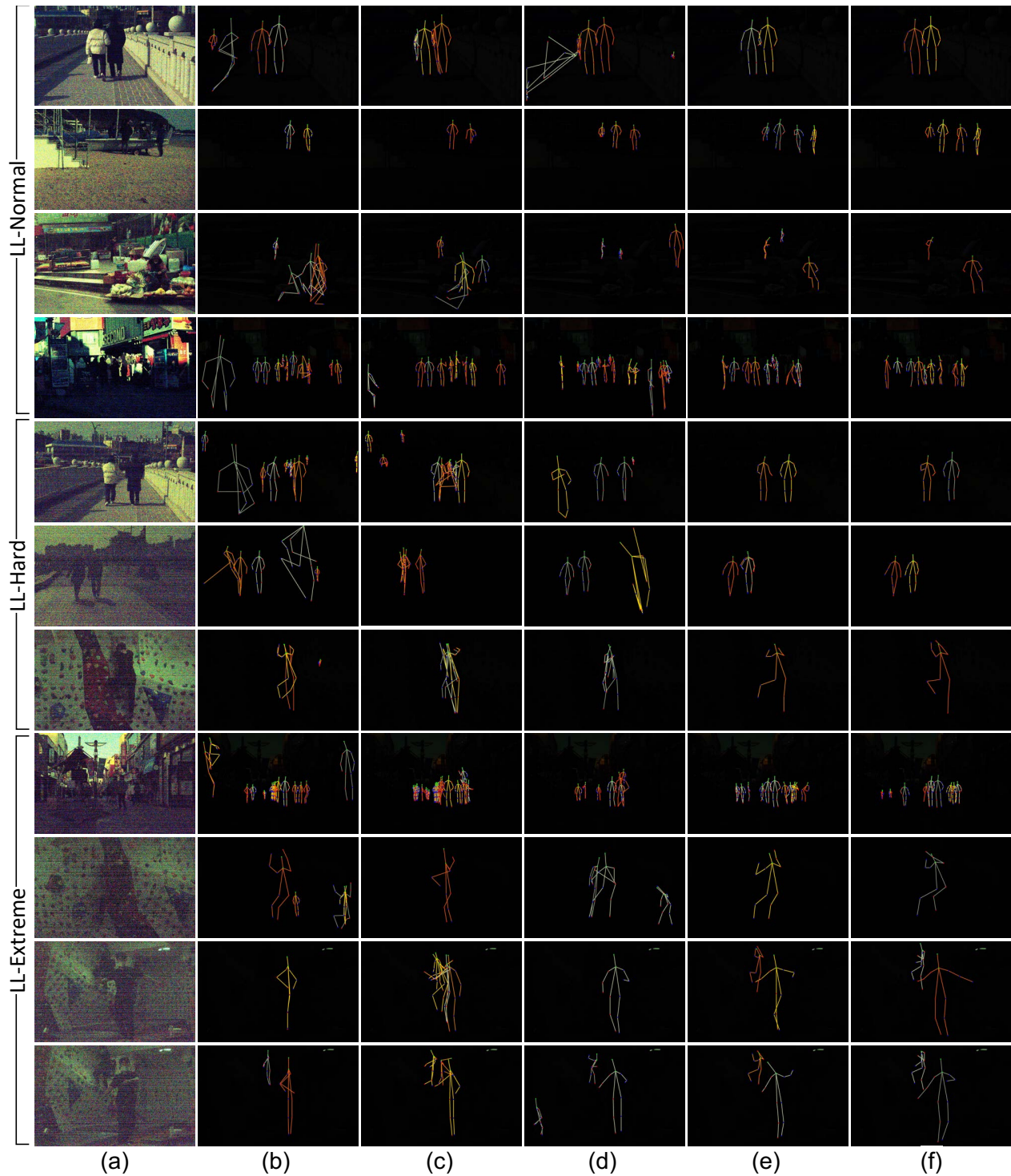
Figure a14. Qualitative results for multi-person pose estimation on the ExLPose dataset. Predicted poses and labels are visualized on corresponding low-light images. (a) Scaled low-light images. (b) Baseline-all. (c) DANN. (d) LIME + Baseline-all. (e) Ours. (f) Ground-truth.
